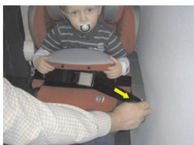
Tighten the belt by pulling the loose end.
