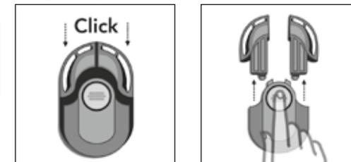
You can position the shoulder harnesses at 3 levels. Always use the position closest to the shoulder level of your child. To open the harness press the central button on the buckle. To adjust the shoulder/ waist harness pull the free ends of the strap.
