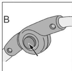
Press and hold the adjustment buttons on both sides and adjust the height of the handlebar to the desired position.
