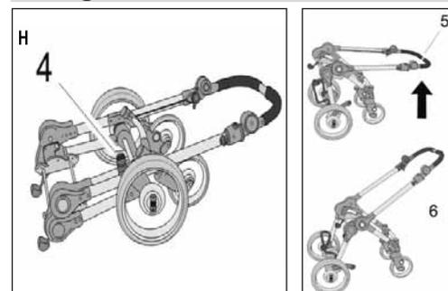
Disengage the transport lock (4) and use the swiveling handlebar (5) to unfold the pushchair until it audibly clicks into the depicted position (6).
