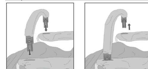
Push the insert pieces on the safety bar through the slots in the seat cover into the receptacles beneath, which are located in the armrests. Make sure that the safety bar has clicked into place on both sides. To remove it, press the release buttons on the insert pieces. In order to make it easier for your child to get in and out, it suffices to release and fold up one side of the bar.
