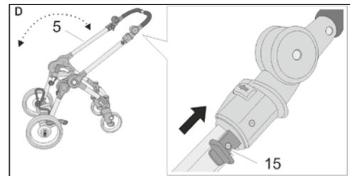
Pull and hold the arrester on the swiveling handlebar (15) in arrow direction; the swiveling handlebar can now be moved to the other of the two positions.
