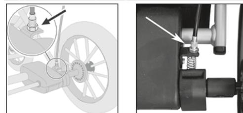
If you should notice a change to the braking action, loosen the lock nut first in order to be able to implement settings on the adjusting screw (unscrew). Then re-attach the lock nut.
