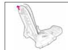
Pull up on the arrester of the back rest to change its inclination angle (4 seating and prostrate positions + folding position all the way forward).
