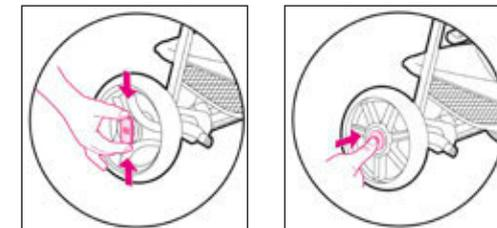
To attach push the wheel onto the axle. Check that the wheel is properly locked by pulling!
