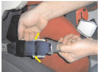
Roll the belt shortener up once more and thread the fixed end of the belt in front of the free hooks.
