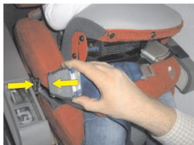
Attach the belt extender to the belt fixed to the seat.
