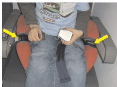
Feed both ends of the lap belt through the belt guides of the child car seat.
