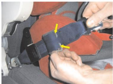
Roll the belt shortener up and thread the loose end of the belt behind the free hooks.
