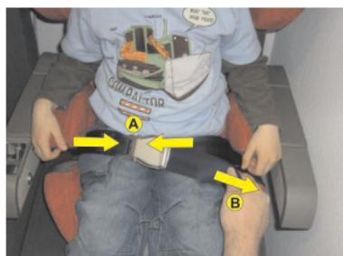
Now close the belt buckle (A) and tighten the belt (B).
