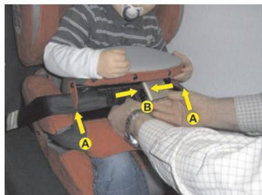
Feed the belt through the impact shield belt guides (A) and close the belt buckle (B).
