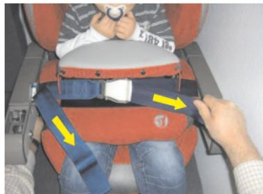
Tighten both loose belt ends. Position the belt buckle in the centre of the impact shield, so that it is easily accessible.
