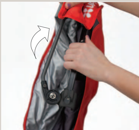
STEP 4: Remove frame from canopy by sliding fabric off of both aluminum and plastic frames.
