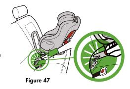
• Pull on LATCH Connector to check that it is securely locked on the vehicle LATCH anchor.
