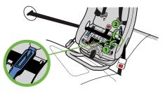
Check that the entire lap/shoulder belt (both the lap and shoulder portions of the belt) is through the Rear-Facing Belt Lock-off being used and under all four Belt Tabs as shown in **Figure 60**. Close-up of Belt Tabs is shown in **Figure 60a**.
