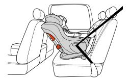
• The top of the child's head must be at least 1" (2.5 cm) below the top of the car seat's Headrest, as shown in **Figure 1**. If the top of the child's head is less than 1" (2.5 cm) below the top of the Headrest in the highest adjustment position, your child is too large for using this car seat Rear-Facing and must be transitioned to Forward-Facing use with this car seat.
